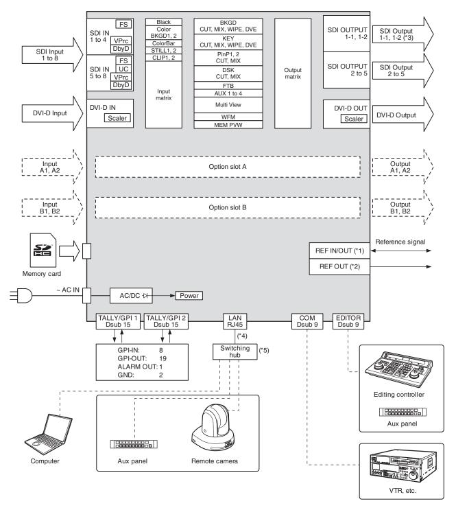
\*1: When external synchronization is selected as the reference signal setting, the reference signal is input.
