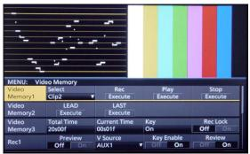
The image display and the WFM display (or VECTOR display) displayed in the upper portion of the built-in display can be switched by pressing the [PICT] button or the [WFM/VECT] button.
