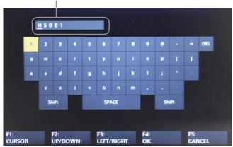
When the keyboard screen is displayed, use rotary encoders [F1] to [F5] to input the characters (alphanumerics and symbols).
